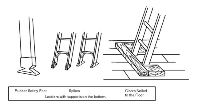
Portable ladders must be used at such a pitch that the horizontal distance from the top support to the foot of the ladder is about one-quarter of the working length of the ladder.
