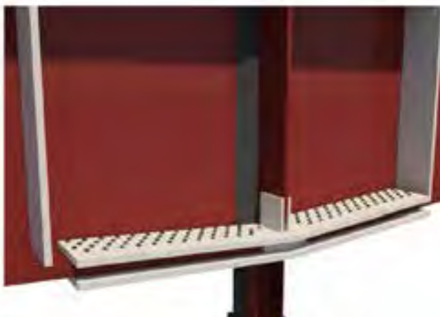
4. Bolted sandwich plate repair
