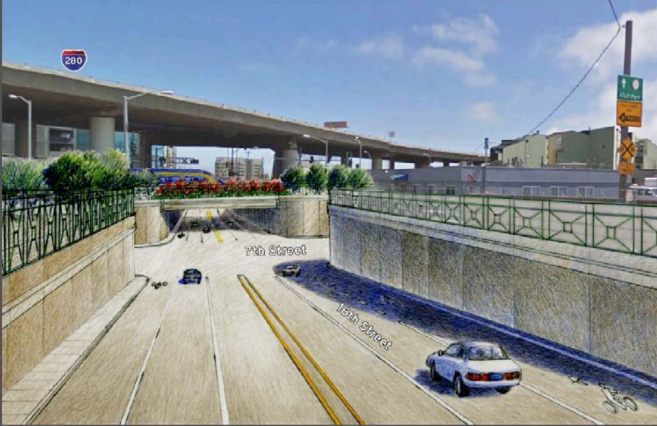
Potential Grade-Separation of 16th Street
