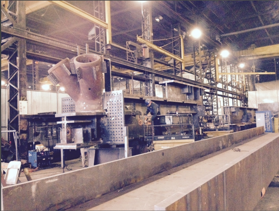
Above and Right : Connection of ground level cast node to transfer girder.
