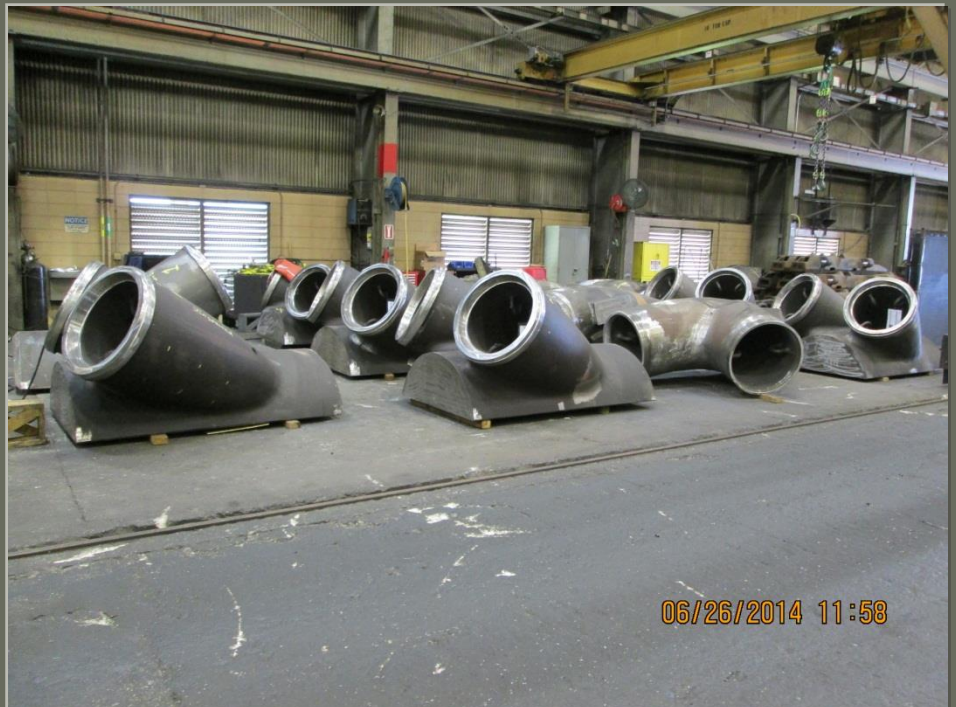
Various node types ready for final inspection.
