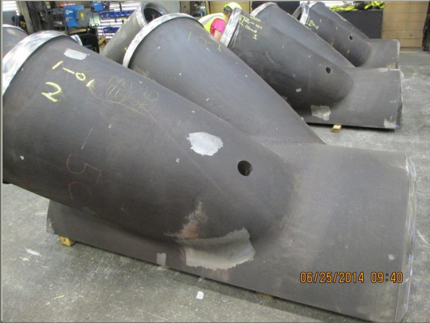
Node Type 1, machining completed, ready for inspection and shipping.
