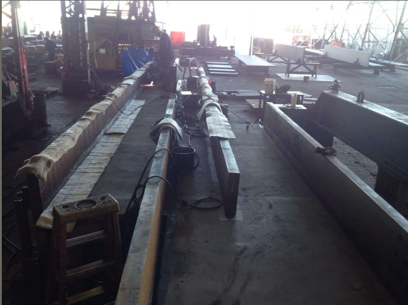
Oregon Iron Works – Built up beam in progress
