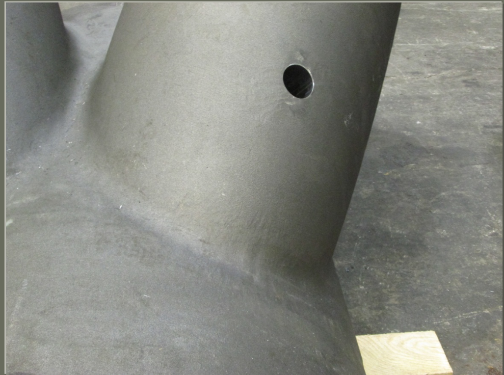
Finished Cast Node Surfaces
