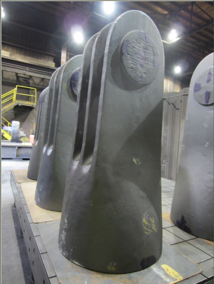
Type 71 and 72 Cast Nodes in Bradken's Kansas Foundry, preliminary cleaning and shot blast complete.
