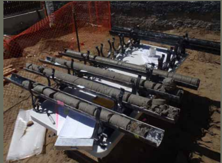
CDSM Shoring Wall Cores
