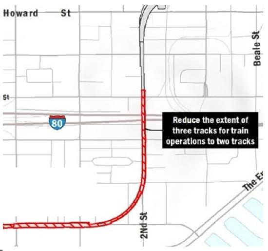
REDUCTION in trackwork portion of tunnel from three to two tracks, enabling smaller tunnel and fewer underground easements for the rock dowels that extend from the tunnel
