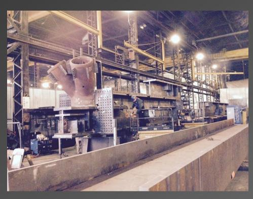
Above and Right: Connection of ground level cast node to transfer girder.
