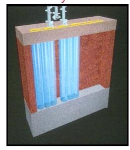
3) Mixing of Secondary Panel Between Two Primary Panels
